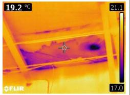
3. Review of the mechanical room penetrations was conducted. Two of the exhaust vents, one from the furnace and one from an HRV was observed with active dripping of water. *Postscript: It is unclear from review of the tender documents if the HRV or furnace*
